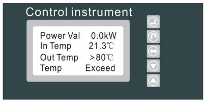
5.If system has no water or water pump does not run, the instrument will automatically enter the alarm state, interlocking is disconnected, the buzzer alarms at the same time, and screen displays the followings:
